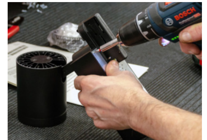
Salvaged components cleaned and reassembled with new LED module, driver and reflector
