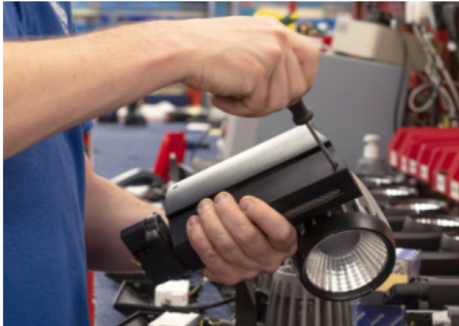
Each luminaire was disassembled and inspected
