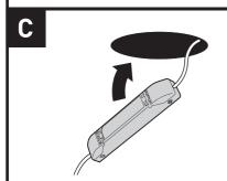
Install driver into ceiling void.
