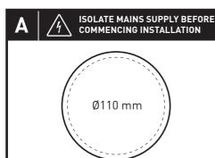
Cut a 110 mm circular hole at desired location
