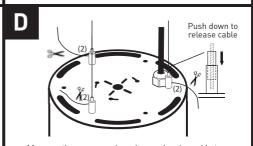
Measure three suspension wires and mains cable to required length and carefully trim.
