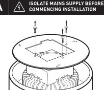
Remove the three screws to lift off the pendant plate.
