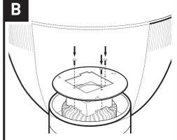
Fit refractor and re-attach pendant plate with screws.
