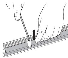
Disconnect the driver connectors and the earth spade to release the LED tray.
