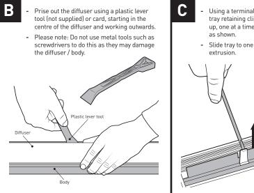
Using a terminal driver, ease out the LED tray retaining clips, whilst pulling the tray up, one at a time and remove the LED tray
