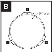
Remove 3 x fixing screws and remove diffuser.
