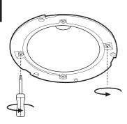
Turn two fitting screws clockwise to secure luminaire into ceiling. DO NOT USE POWER TOOLS.
