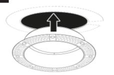
Fit the plaster-in collar into the hole.
