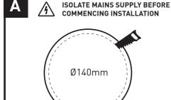
Cut a Ø140mm circular hole at the desired location using a holesaw.
