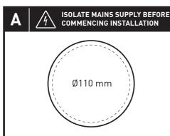
Cut a 110 mm circular hole at desired location
