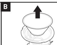
Remove reflector from luminaire taking care not to damage the reflector's surface.
