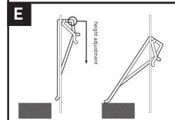
Lock the luminaire in place by means of the four adjustable fixing springs as illustrated above.
