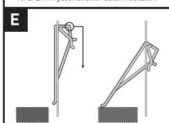
Lock the luminaire in place by means of the four adjustable fixing springs as illustrated above.
