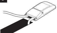
Feed the driver into the ceiling void, ensuring it is not covered by any debris or insulating material and is correctly positioned.
