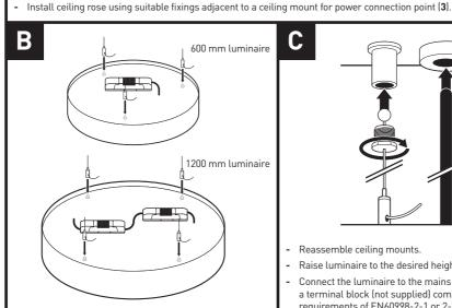
Screw suspension clutches on to studs on the back of luminaire. Three suspension clutches for 600 mm luminaire or four for 1200 mm luminaire.
